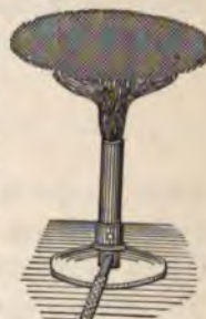
FIG. 192. — Illustrating the principle of the Davy safety lamp.
